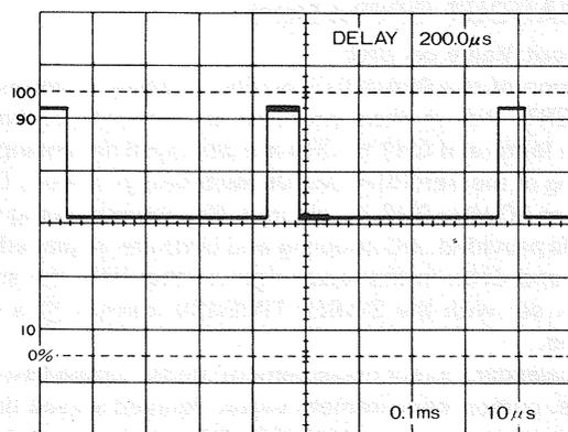
Though the delay time, 200 $\mu$ s, is set at the point of 2 div., the trigger point after it is at the point of 4.3 div.; consequently, the part from 4.3 div. is intensity-modulated (for magnification).
