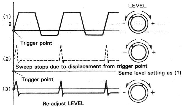
(b) In case trigger level is set on negative side of waveform (NORM)
